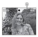
When the jitter alert appears, we recommend using a tripod. If you cannot use a tripod, be careful of how you hold the camera. (P32)
